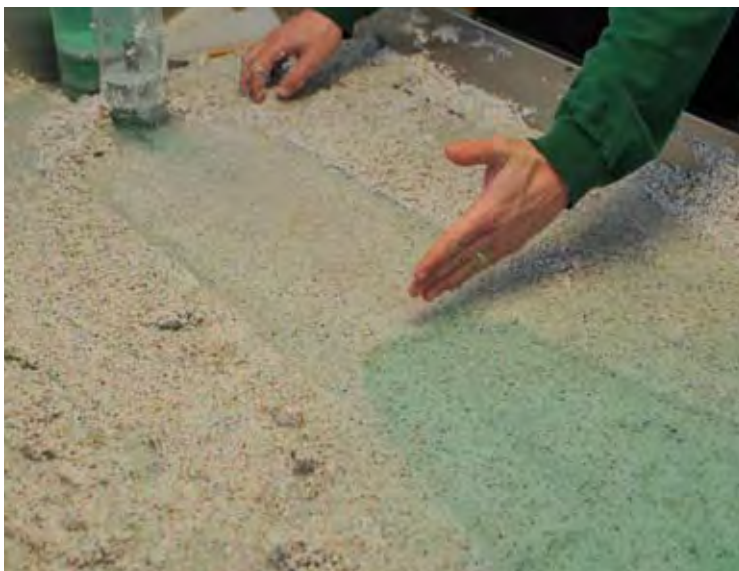
Deposition occurs at the upstream end of the impoundment as demonstrated in the Huron Pines River Model.
