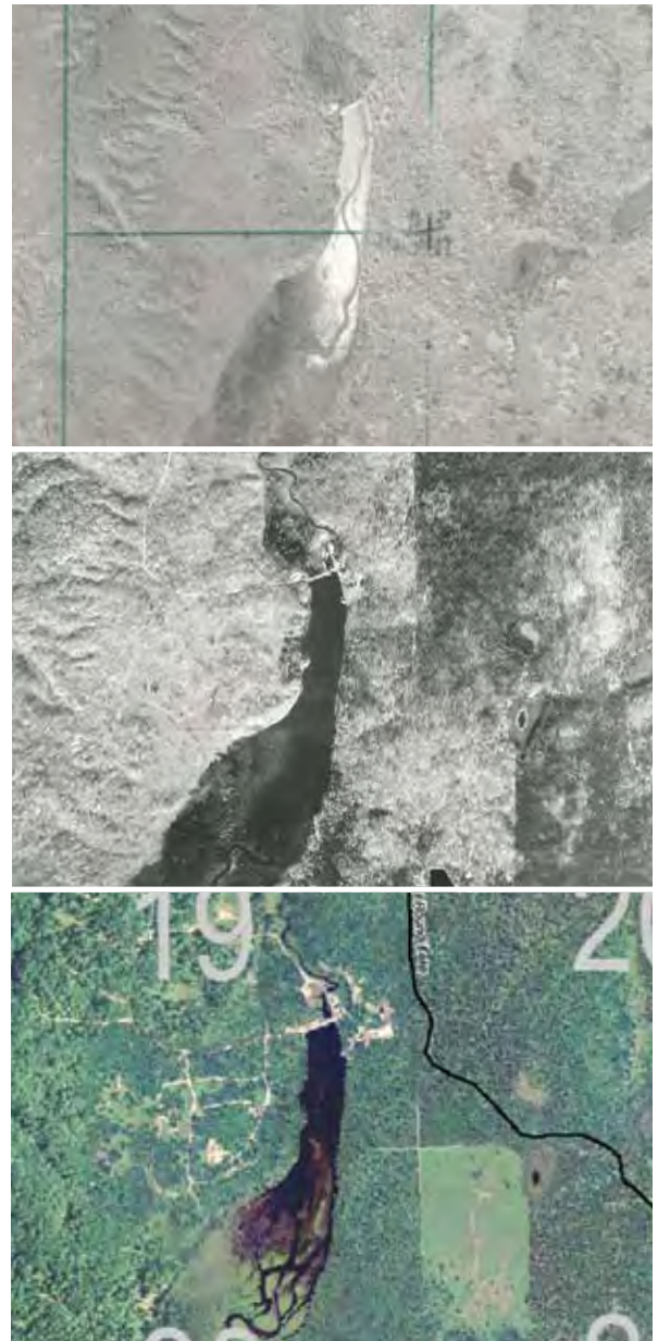
Aerial photos of the same dam in 1938, 1963 and 2005 show how the sediment deposition in the impoundment causes subsequent braiding of the channel.
