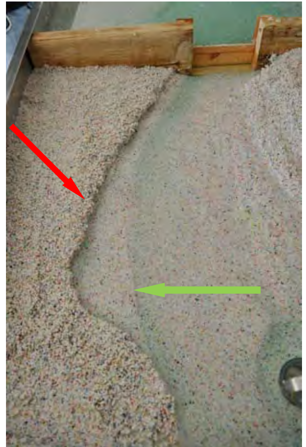
An overhead view of a river "mining" sediment downstream from a dam as the river incises. The red arrow depicts the streambank before the dam. The green arrow shows the development of the new streambank, or terrace.
